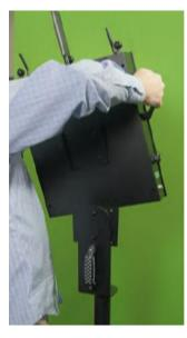
Guard-Dog supports an optional portable stanchion allowing the unit to be easily moved and placed into temporary security setups without access to AC power for instance. Simply slide the back of the unit onto the mounting plate included with your optional stanchion pole. Use long а screwdriver to fully secure the unit to the stanchion mount.
