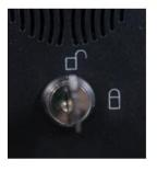
**Guard-Dog** includes a provision to securely lock all settings with a physical key to prevent tampering. Settings such as thresholds, alerts and even power may not be changed while the **Guard-Dog** is locked. In addition, **Guard-Dog's** touch screen requires a six digit PIN code in order to make any changes using the touchscreen even while the unit is physically unlocked.
