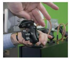
**Guard-Dog** supports an optional direction finding antenna kit including 2 dual band directional antennas to cover both 2.4 GHz and 5 GHz, 1 wideband directional antenna covering 700 MHz to 2.7 GHz, mounting brackets and cables. Simply unscrew the SMA mounted omni-directional antennas that are included with your unit and replace them with the directional antennas. Be sure
